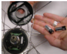
Figure 12: Hub Battery replacement
