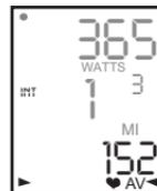
In trip mode "INT" and the new interval number will appear and disappear (FIGURE 26). The computer can mark an unlimited number of intervals although after nine (9) the marker will begin to count back at one (1). For example, interval ten (10) is displayed following interval (9) as one (1).
